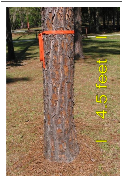
The Diameter at Breast Height (DBH) is measured at 4½ feet above the ground.
